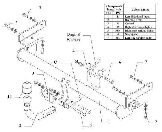
This towbar is designed to assembly in following car: MITSUBISHI CARISMA 4/5 door (DA), produced since 07.1995 till 06.2006, catalogue number Z23 and is prepared to tow trailers max total weight 1450 kg and max vertical load 75 kg.
